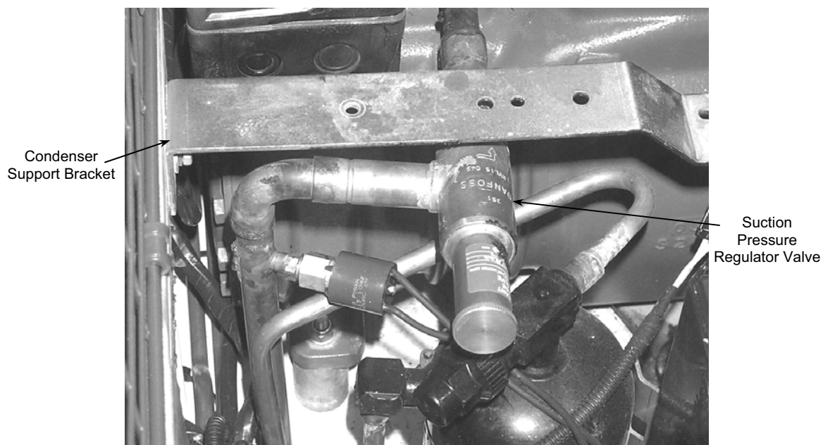
Figure 1. Suction Pressure Regulator Valve.
